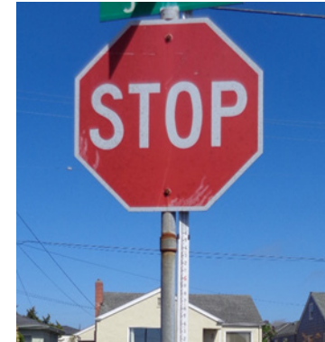
A sign which failed the retroreflectivity test.
