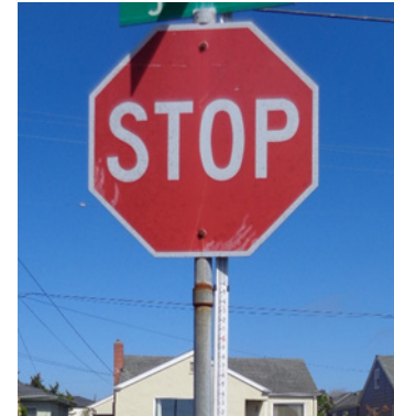
A sign which failed the retroreflectivity test.
